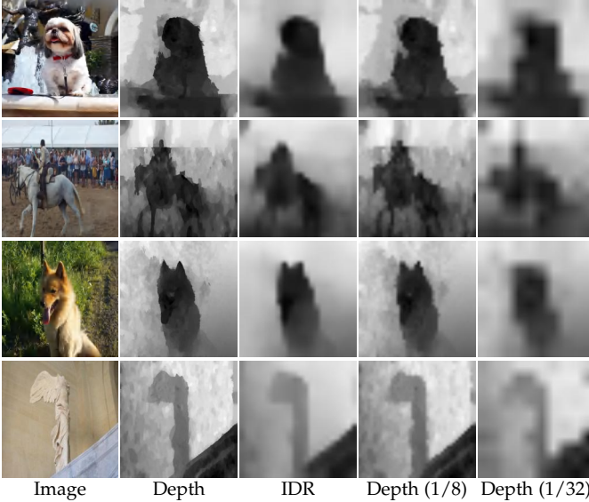
Figure 5. Visual comparisons of restored depth maps by IDR with different scales of input depth maps. Results of the last 3 columns have been upsampled with bilinear interpolation to match the size of the input depth map.
